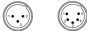
DMX 512 XLR plug (male) Front view of the plug
