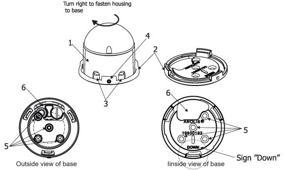
1. Fasten the ArcDot's base (2) on the mounting surface. Keep its orientation as shown on the picture above (sign DOWN has to lead down).
